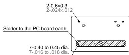
Tolerance:  $\pm 0.1 \pm 0.004$ General tolerance:  $\pm 0.3 \pm 0.012$
