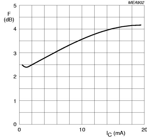
$V_{CE} = 5$  V;  $Z_s = 60$  Ω;  $f = 800$  MHz;  $T_{amb} = 25$  °C.
