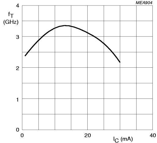
$V_{CE} = 5$  V;  $f = 500$  MHz;  $T_{amb} = 25$  °C.
