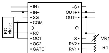
Output can be turned on or off by adding a signal of the TTL level between the RC terminal and the COM terminal or by releasing the connection between the terminals.
