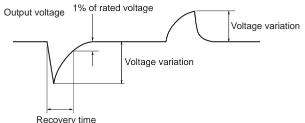
The voltage variations depend upon conditions of the input voltage and the load current.
