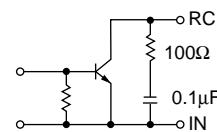
1 For the SPL type, the rise time or the fall time of a signal to the RC terminal should be 2ms or shorter.
