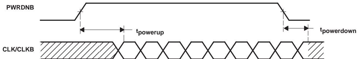
Figure 8. PWRDNB Transition Timings
