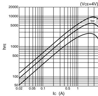
$h_{FE}$ - $I_c$  Temperature Characteristics (Typical)
