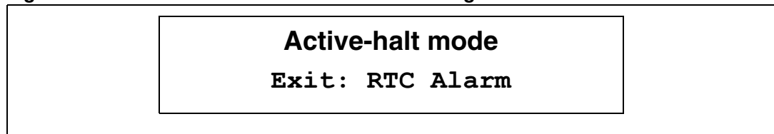
Figure 29. Exit from Active-halt with alarm message
