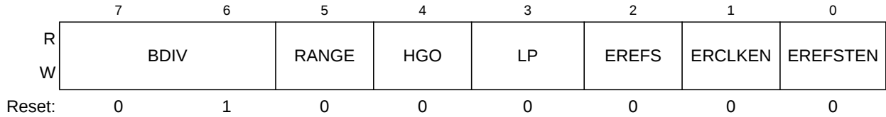
Figure 10-4. ICS Control Register 2 (ICSC2)
