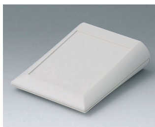
A0612007 COMTEC 120 F, Vers. I ABS (UL 94 HB) off-white RAL 9002 4.72"x5.91"x1.69" IP 40
