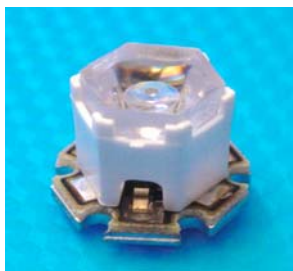
128 Holder and 120 Optic mounted on 3W Luxeon Star PCB
