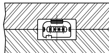
(Note.) For MQ172, mounting to circuit boards is SMT type.
