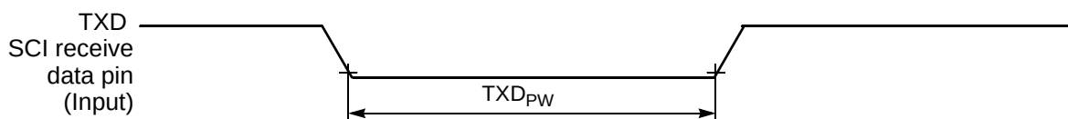
Figure 3-25 TXD Pulse Width
