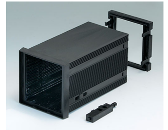
B6023061 DIN-MODULAR CASE TYPE A PPO (UL 94 V-0) black RAL 9005 2.83"x2.83"x4.88"
