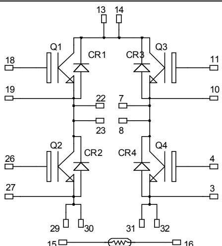
Top switches : Trench + Field Stop IGBT3
