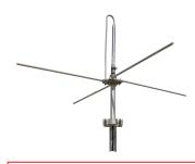
1-port omni ground plane antenna, 144–174 MHz, 360° HPBW, fixed electrical tilt. Bandwidth: 2% of frequency.
