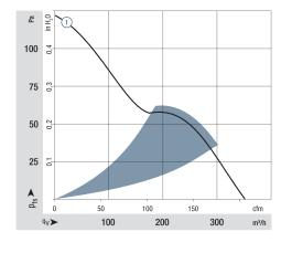
Air performance measured according to: ISO 5801. Installation category A, without contact protection. Noise: Total sound power level  $L_WA$  ISO 103002 measured on a hemisphere with a radius of 2 m. Sound pressure level LpA measured at 1 m distance from fan axis.
