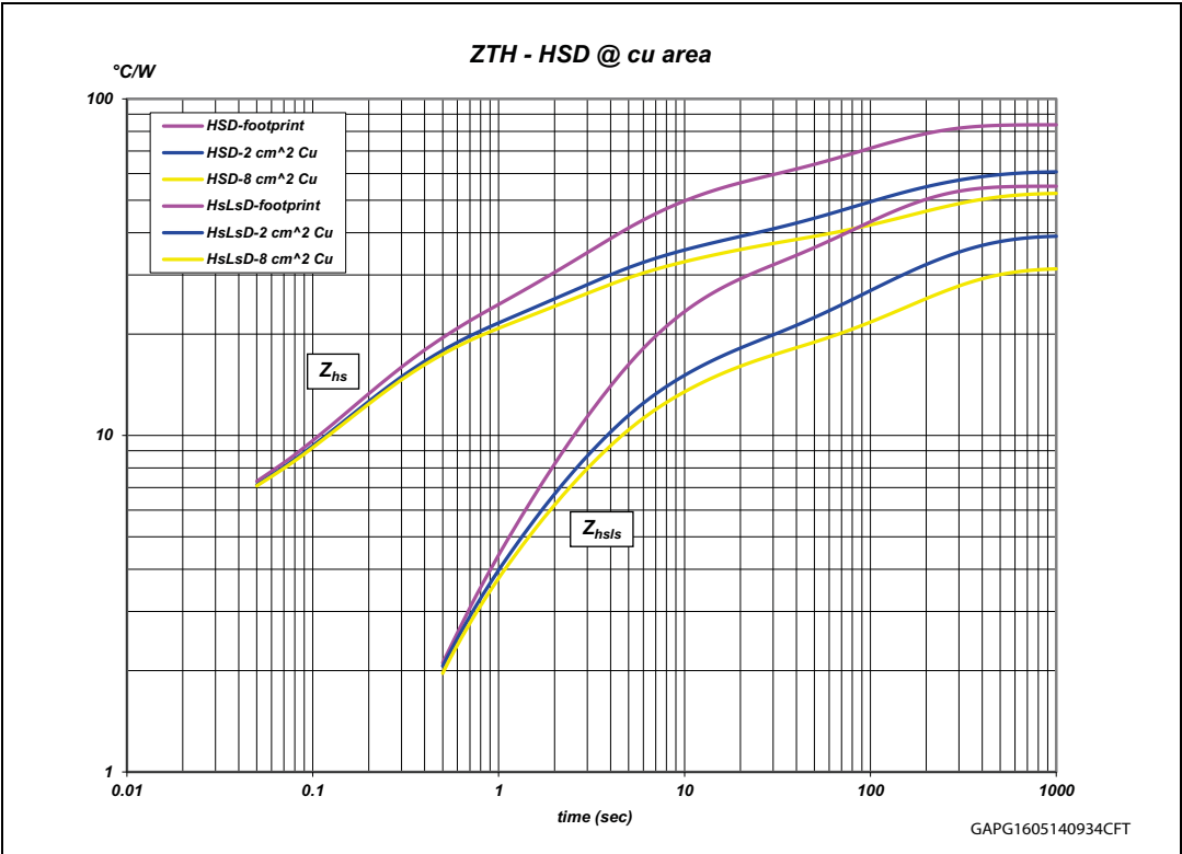
Figure 17. HSD thermal impedance junction ambient single pulse
