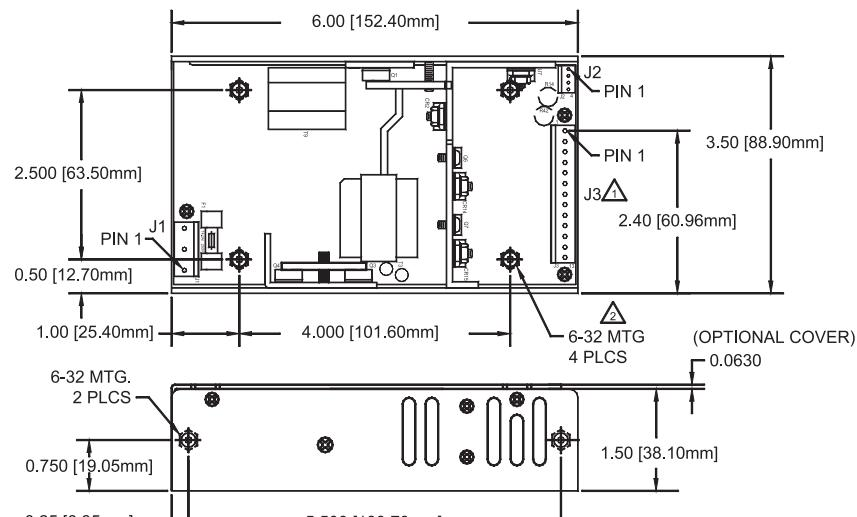
▲ 5A MAXIMUM RECOMMENDED CURRENT PER CONNECTOR PIN, WITHOUT AIR.
