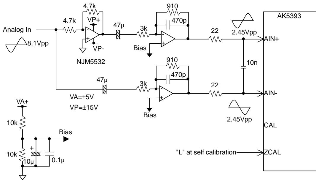
Figure 7 Differential Input Buffer Example
