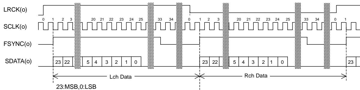
Figure 2. Serial Data Timing (Master mode, DFS="L")
