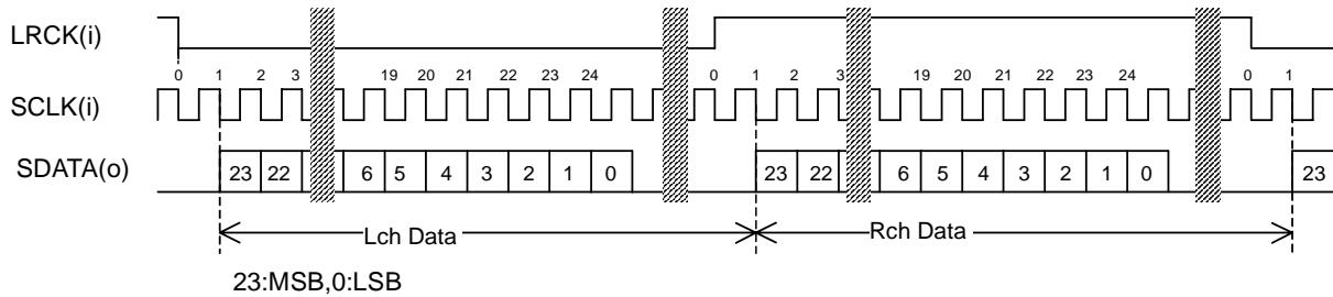
Figure 3. Serial Data Timing (I<sup>2</sup>S Slave mode, FSYNC: Don't care.)
