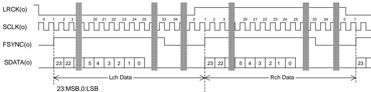
Figure 4. Serial Data Timing (I<sup>2</sup>S Master mode, DFS="L")
