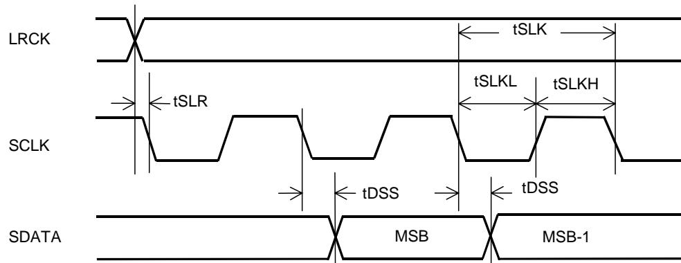
Serial Data Timing (I<sup>2</sup>S Slave Mode,  $\text{FSYNC} = \text{Don't Care}$ )
