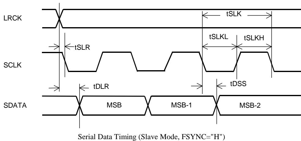
Serial Data Timing (Slave Mode,  $\text{FSYNC} = \text{"H"}$ )
