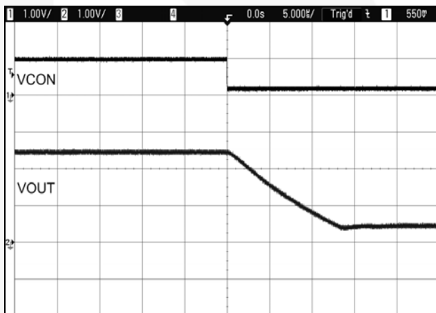
Figure 37. V_{OUT} Falling Transition 2.5 V to 0.5 V, V_{IN} = 3.7\text{ V} in Low-Power Mode
