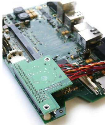
Fig. 4 LVDS Converter installed on Orchid
