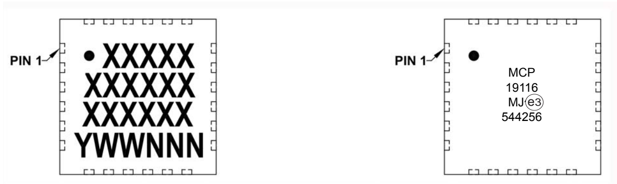
24-Lead QFN (4x4x0.9 mm) ( MCP19116 only )
