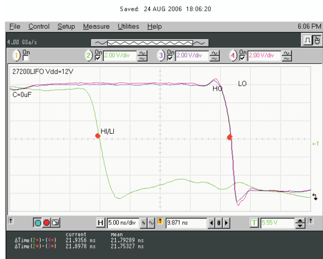
Figure 32. V_{LO} and V_{HO} Falling Edge Delay Matching
