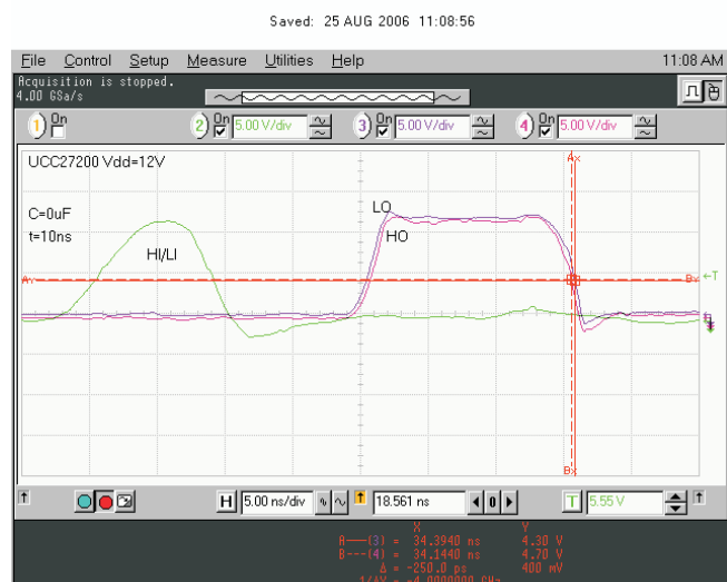
Figure 34. 10-ns Input Pulse Delay Matching
