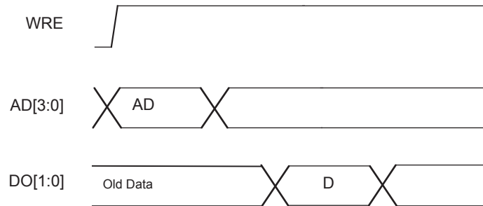
Figure 3-7. Slice Single /Dual Port Read Cycle Timing
