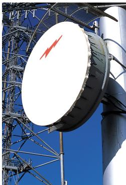
2.4 m | 8 ft High Performance, Super High XPD Parabolic Shielded Antenna, dual-polarized, 7.725–8.275 GHz, PDR84, gray antenna, enhanced white radome with flash, standard pack—two-piece reflector
