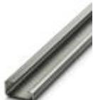
G-profile DIN rail, material: Steel, unperforated, height 15 mm, width 32 mm, length 2 m
