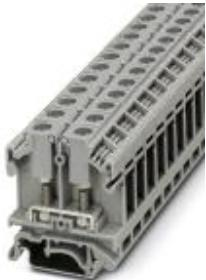
Bolt connection terminal block, Connection method: Bolt connection, Cross section: 0.1 mm<sup>2</sup> - 6 mm<sup>2</sup>, AWG: 26 - 10, Width: 11 mm, Color: gray, Mounting type: NS 35/7,5, NS 35/15, NS 32
