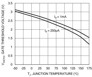
Figure 8. Gate Threshold Variation vs. Temperature
