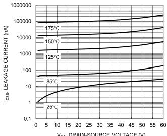
Figure 10. Typical Drain-Source Leakage Current vs.
