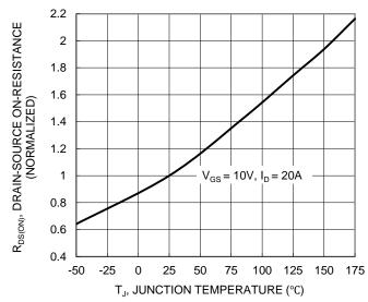
Figure 6. On-Resistance Variation with Temperature
