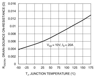
Figure 7. On-Resistance Variation with Temperature
