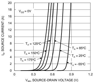
Figure 9. Diode Forward Voltage vs. Current
