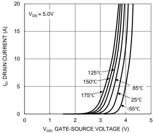
Figure 2. Typical Transfer Characteristic
