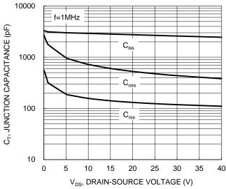
Figure 11. Typical Junction Capacitance
