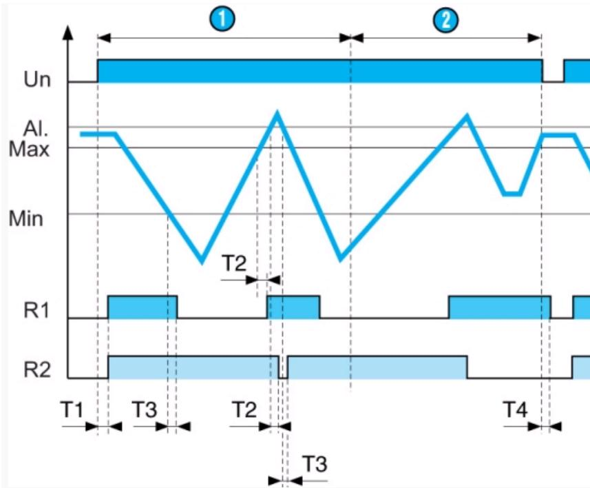
On power-up, probes Min, Max are submerged and probe Al. is above the level of the liquid. Relays R1 and R2 are energised and the pump is ON : emptying starts, the LED for relay R1 is lit. When the Min probe emerges, relay R1 de-energises and the pump if OFF : emptying stops, the LED for relay R1 goes off. If, in the event of a fault, the level continues to rise and reaches probe Al., relay R2 de-energises and the alarm is triggered : the LED for relay R2 is lit. This fault can be stored.
