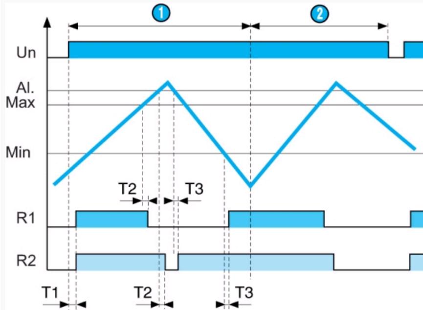
On power-up, the level in the tank is low, relays R1 and R2 are energised and the pump is ON : filling starts, the LED for relay R1 is lit. When the level reaches the Max probe, relay R1 de-energises and the pump is OFF : filling stops, the relay LED goes off. If, in the event of a fault, the level continues to rise and reaches probe Al., relay R2 de-energises and the alarm is triggered : the LED for relay R2 is lit.
