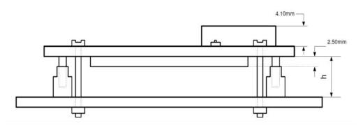
h represents the base board connector height (minimum 5mm) and its value needs to be chosen in such a way that ensures: 2.5mm + 4.1mm +  $h \le 13.7$ mm.
