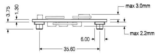
The module measures  $60 \times 44$ mm. Two holes are provided for M2 screws to enable secure mounting of the module on the base board.
