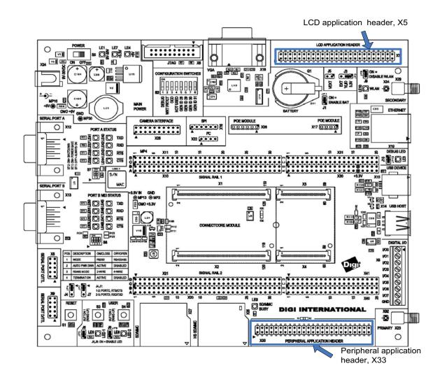
The development board provides two, 2x25-pin, 0.10" (2.54mm) pitch headers for supporting application-specific daughter cards/expansion boards:
