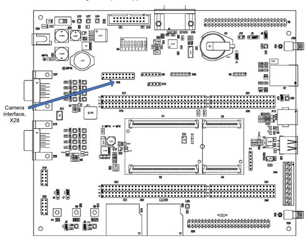
The camera interface signals are provided on a 2x10 pin header including the I2C bus. The Digi Multimedia Application Kit (Digi P/N CC-ACC-MMK-2443) provides a camera sensor reference design. Please contact your distributor or Digi sales office for details.
