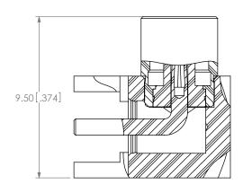
IN-PROCESS 4 ATTACH SHELL TO BODY
