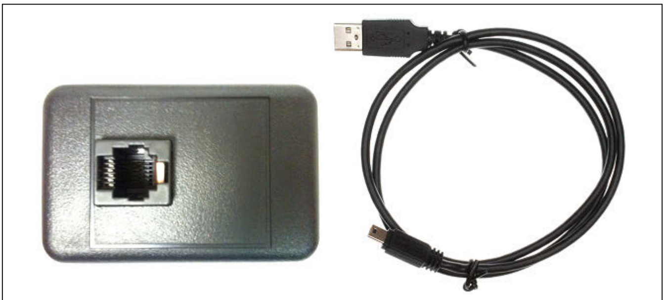
Figure 1. DS9481R USB-to-1-Wire/iButton Adapter and Cable
