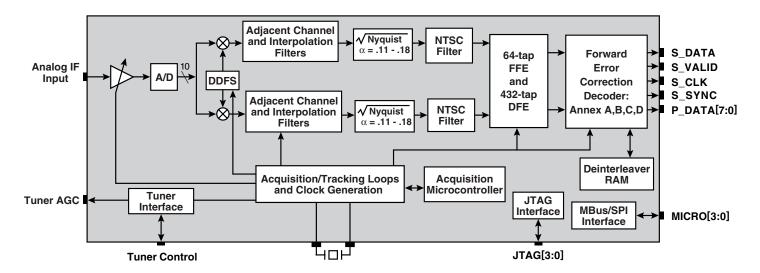
The Broadcom BCM3510 is a VSB/QAM digital receiver, compatible with both North American digital cable television and digital terrestrial broadcast television standards. The BCM3510 is capable of receiving all Standard-Definition and High-Definition digital television formats (SDTV/HDTV).
