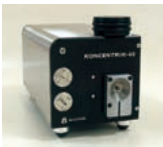
Ferrule concentricity + index measurement
