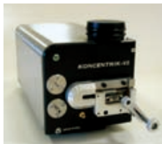
Patchcord concentricity + index measurement
