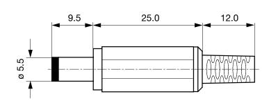
Cable diameter max. 4.0 mm
