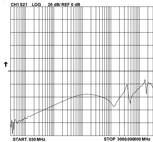
ESD Clamping (15kV Air)
