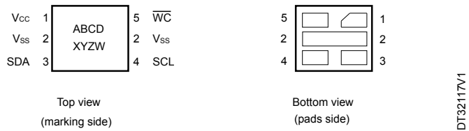
Figure 3. UFDFPN5 (DFN5) package connections
