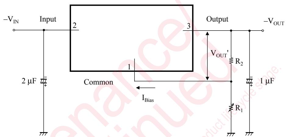
$$|V_{OUT}| = V_{OUT}' \left( 1 + \frac{R_1}{R_2} \right) + I_Q R_1$$
