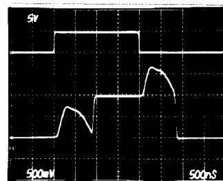
MUX-24 SMALL-SIGNAL SWITCHING WITH 2μs SAMPLE TIME
