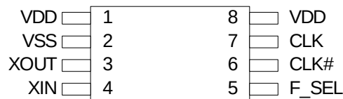
Figure 1. Pin Diagram - 8 Pin TSSOP
