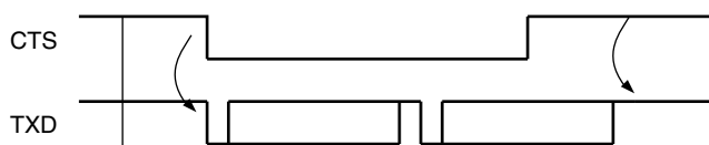
Figure 39-28. Transmitter Behavior when Operating with Hardware Handshaking
