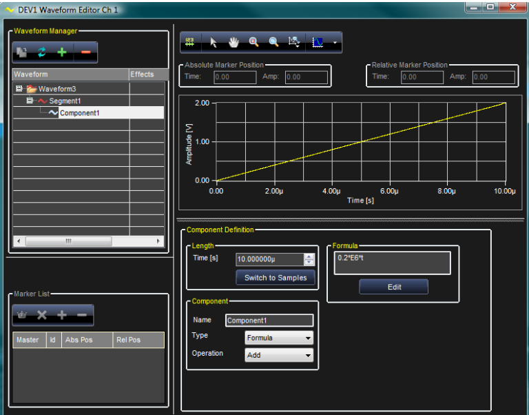
A ramp waveform. The actual formula used here is 0.2*E6*t. Set the time to 10.000000μ to view the graph as previously shown.
