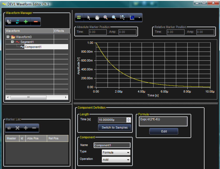
A decaying exponential waveform. The actual formula used here is \text{Exp}(-t/(2 \times 10^{-6})) . Set the time to 10.000000 μs to view the graph as previously shown.
