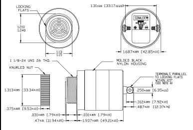
NOTE A: TERMINALS-032 BRASS TIN PLATED, TAPPED FOR #6-32 SCREW. TWO #6-32 NICKEL PLATED BRASS SCREWS INCLUBED. WILL ACCEPT 1/4' QUICK CONNECT. NOTE B: MOUNTING- REMOVE BLACK PLASTIC NUT AND INSERT THREADED FRONT THROUGH 1.25' HOLE PUNCHED IN PANEL, IF DRIENTATION IS NEEDED, NOTE LOCKING FLATS ON DRAVING. SCREW NUT BACK ON. DO NOT OVERTIGHTEN.
