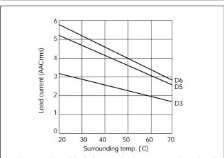
Derating curve is used for finding max. load current at an elevated ambient temperature. The 3 lines in the graph represent the 3 nominal current ratings of the RP1 series (RP1...D3/D5/D6).
