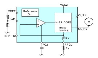
The output response time depends on the FC2 capacitance and interval of Input signal because there is no FC quick charging circuit in current drive2.
