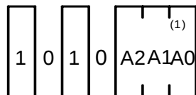
Figure 44. Difference of Slave Address of Each Type
