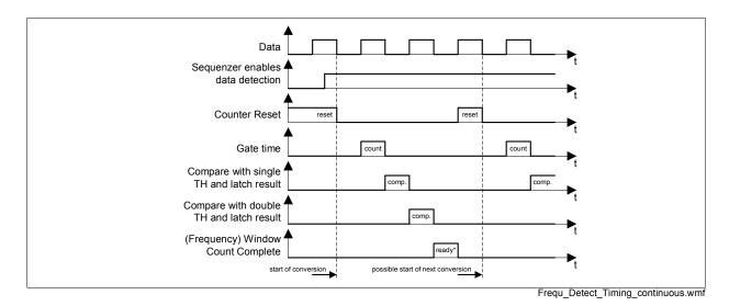
Figure 3-28 Frequency Detection timing in continuous mode
