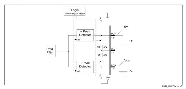
Figure 3-26 Peak detector - power down mode
