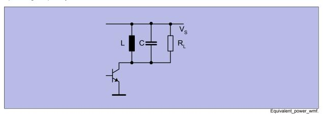
Figure 3-6 Equivalent power amplifier tank circuit
