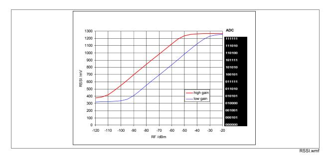
Figure 3-21 Typ. RSSI Level (Eval Board) @3V
