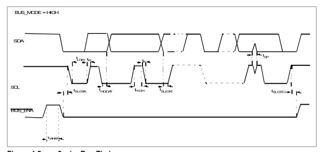
Figure 4-2 3-wire Bus Timing
