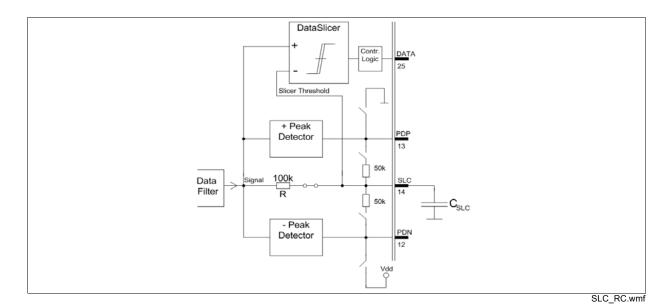
Figure 3-22 Slicer Level using RC Integrator
