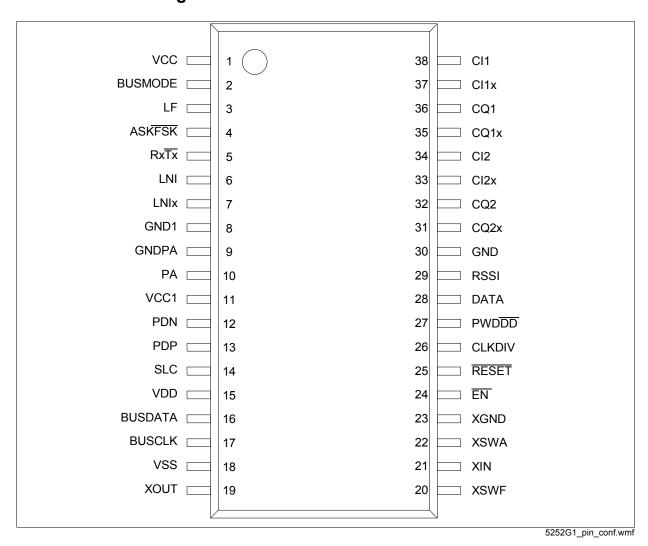
Figure 2-1 Pin Configuration
