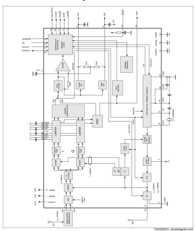
Figure 2-2 Main Block Diagram
