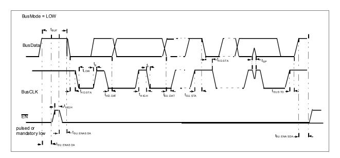
Figure 4-1 I<sup>2</sup>C Bus Timing
