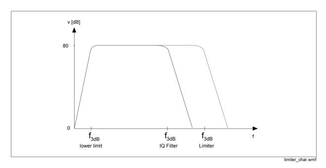
Figure 3-20 Limiter frequency characteristics
