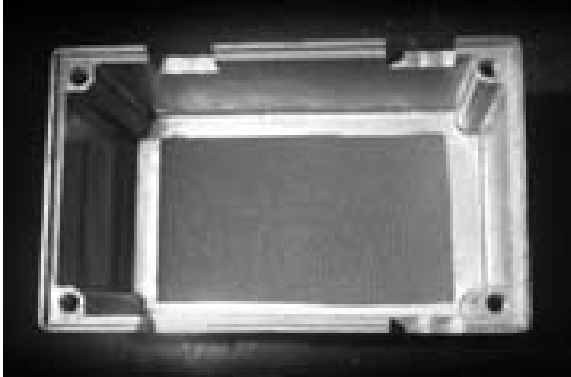
Figure 3. Enclosure with Q-Zorb PN 2238 Installed
