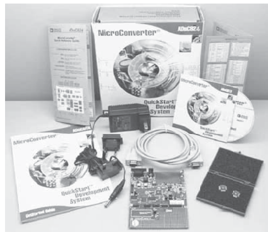
Figure 47. Components of the QuickStart Development System
