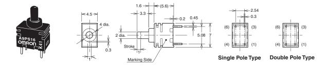
Note: NO.(4) and (6) terminals in the Single Pole models are dummys to support the Switch case.
