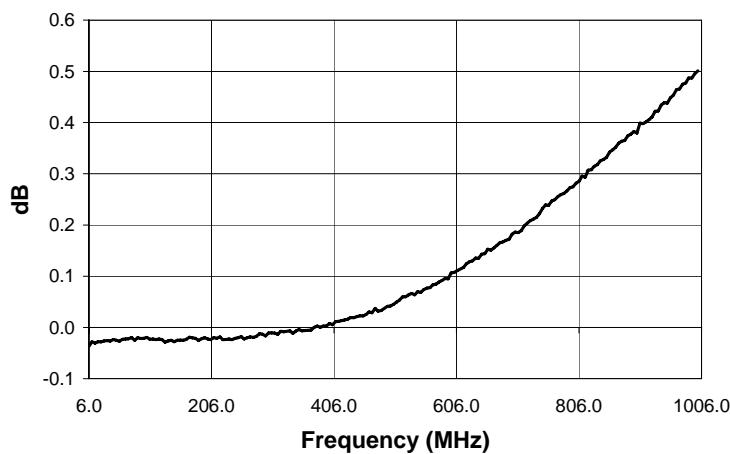
**E-Series RF 1:4 Transmission Line Step-up Transformer**
