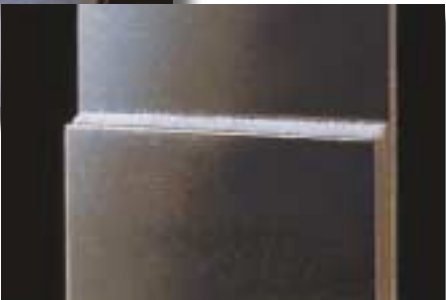
Under equal stress conditions, metal panels bonded with VHB tape show no visible signs of stress compared to those with mechanical fasteners.
