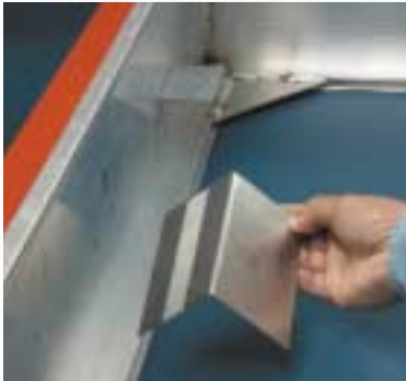
Permanently attach brackets and stiffeners.
